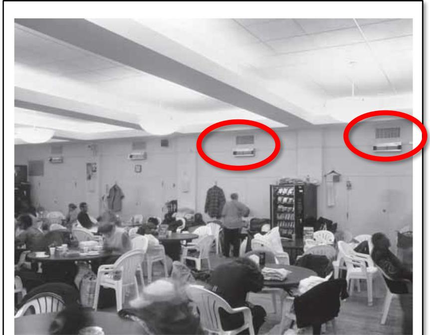
Tuberculosis Ultraviolet Shelter Study New York City shelter in a church basement. Note the ultraviolet germicidal irradiation fixtures located on the upper wall, directly below the vents. Photo: ©Randall Perry Photography.
